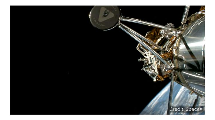
Initially, the star tracker information was numerically conditioned slightly differently than we anticipated. We were expecting a one-in-a-thousand numerical tolerance and received a number more like two and three in a thousand. So, Nova-C's navigation system rejected the star tracker data.
